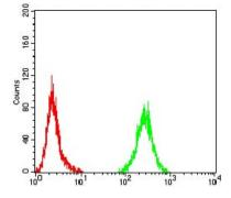
Flow cytometric analysis of Hela cells using PLCG1 mouse mAb (green) and negative control (red).
