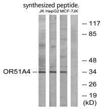
Western blot analysis of lysates from Jurkat, HepG2, and MCF-7 cells, using OR51A4 Antibody. The lane on the right is blocked with the synthesized peptide.
