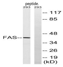
Western blot analysis of lysates from 293 cells, using FAS Antibody. The lane on the right is blocked with the synthesized
