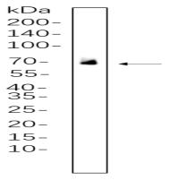
U-14 whole cell lysates were separated by 10% SDS-PAGE, and the membrane was blotted with primary antibody(1:1000).
