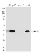
Western blot analysis of PRMT6 in COS7, Jurkat, C6, 3T3 and Hela lysates using PRMT6 antibody.
