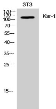
Western Blot analysis of NIH-3T3 cells using Ksr-1 Polyclonal Antibody
