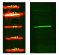
Western Blot analysis of HEK293 lysis, using primary antibody at 1:1000 dilution. Secondary antibody was diluted at 1:10000
