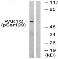
Western blot analysis of lysates from LOVO cells treated with starved 24h, using PAK1 (Phospho-Ser199) Antibody. The lane on the right is blocked with the phospho peptide.
