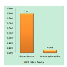
Enzyme-Linked Immunosorbent Assay (Phospho-ELISA) for Immunogen Phosphopeptide (Phospho-left) and Non-Phosphopeptide (Phospho-right), using Cyclin E1 (Phospho-Thr395) Antibody
